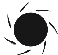
Owl airfoil centrifugal wind turbines
